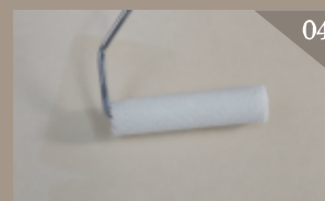
Cover layer (recommended to use seamless cover). Apply evenly twice with a roller add 10-15% water
